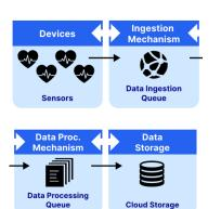
Sensors communicate to the cloud using MQTT via either using WiFi or LTE cell network. No data is lost. All sensor communications can be seen in the cloud for updating firmware, debugging and diagnostics purposes. The system can be scaled to 100,000+ sensors instantly by allocating more resources on the server. The diagram shows the data flow from the sensor to the cloud.
