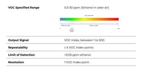
The VOC Index is a robust measure for indoor air quality. It automatically adapts the environment the sensor is exposed to. The VOC Index shows changes of intensity of VOC events relative to the history of the room, referenced to the average of VOCs present over the last 24 hours. The Index doesn't represent absolute concentrations but refers to the typical conditions of the environment. It indicates users when air pollution changes and the room needs to be ventilated or the air purified.
