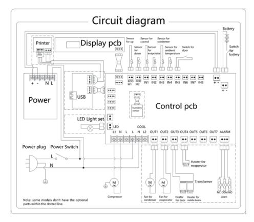
Note: Optional parts are included in the dash-dotted line, and some models are not equipped. Applicable to YC-315/YC-395L/YC-395EL/YC-400L/YC-525L/YC-725L/YC-1015L/YC-1015EL/YC-1505L
